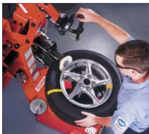
Use the TC3500 to easily and safely rotate the tire on the wheel to eliminate vibration.
